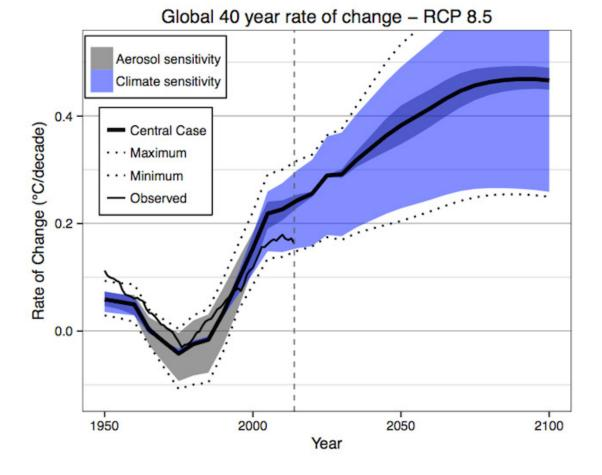
Global rates of decadal temperature change over 40-year periods. Results are shown for: central climate assumptions (thick solid line), range due to uncertainty in aerosol forcing (grey shading), and range due to uncertainty in climate sensitivity (blue shading). The outer bounding cases are shown as dotted lines. The thin solid black line shows the historical rate of change using the HADCRU4 observational data. The vertical dashed line indicates 2014. Via PNNL.
